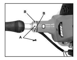
5. Tighten two (2) drive shaft clamp bolts (B) securely.
